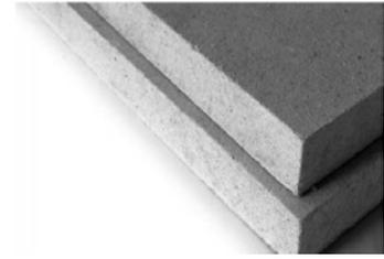
**Knauf Vidiwall is a gypsum fibreboard manufactured from gypsum and cellulose fibres from recycled paper. This dense sheet material is suitable for all areas of drywall construction requiring a dense, impact resistant product capable of providing increased durability, rigidity and mechanical strength compared to a traditional gypsum sheet plasterboard.**
