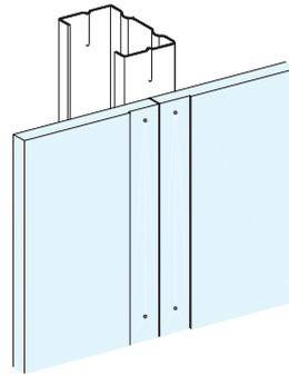
**1** The boards should be closely butt jointed.
