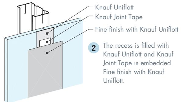
**2** The recess is filled with Knauf Uniflott and Knauf Joint Tape is embedded. Fine finish with Knauf Uniflott.
