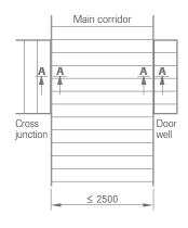
The perimeter wall details in the main corridor should be installed for best optical effect. At corridor cross junctions and in door wells it is also possible to make a perfect transition between the ceiling surfaces. Other junction connections are possible, for example with Bandraster profiles which are extremely rigid and can provide security against pressure and lateral thrust.
