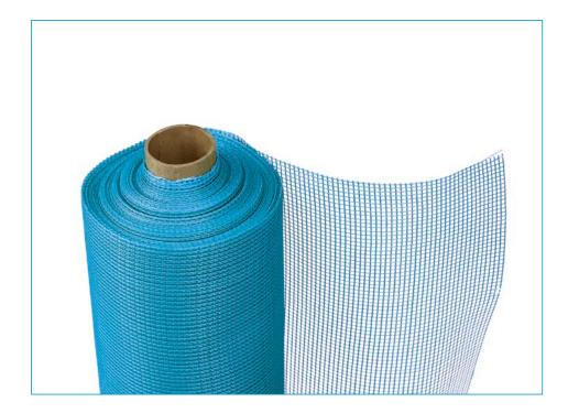
AQUAPANEL® Exterior Reinforcing Mesh is a wide-mesh glass fabric designed to resist sliding. It is manufactured from glass filament fibres with a nominal diameter of < 5  $\mu$ m. AQUAPANEL® Exterior Reinforcing Mesh is used to reinforce AQUAPANEL® Exterior Basecoat and AQUAPANEL® Joint Filler and Skim Coating – White (exterior ceiling applications only).
